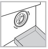
position a container so that it will collect the water which flows out (approximately 1.5 l) (see figure);
